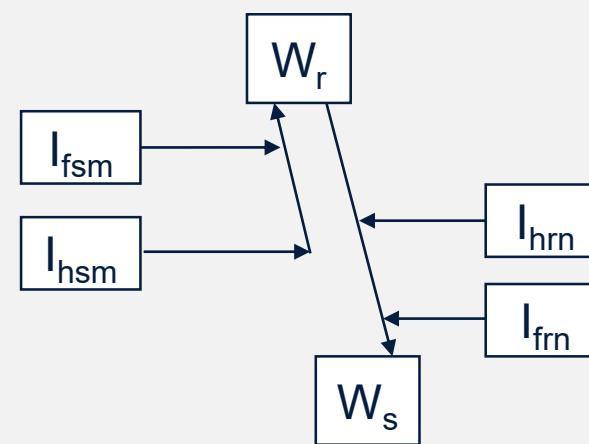
$$\frac{dW_r}{dt} = \alpha_{Wh}(\lambda_{hsm}I_{hsm} - \lambda_{hrn}I_{hrn}) + \alpha_{Wf}(\lambda_{fsm}I_{fsm} - \lambda_{frn}I_{frn}) - \tau W_r$$
